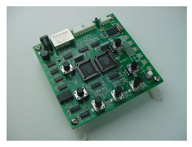
The X-Y Pattern Generator was designed as a test instrument to aid in the repair and alignment of B/W and Color X-Y monitors. This unit cannot be used on Raster scan monitors. The Pattern Generator comes equipped with pass through cable assemblies to fit Wells Gardner 6100 and Electrohome B/W and G08 color X-Y monitors. The unit can be used on other X-Y monitors by building your own cables or ordering custom cables from <a href="mailto:support@vector-labs.com">support@vector-labs.com</a>
