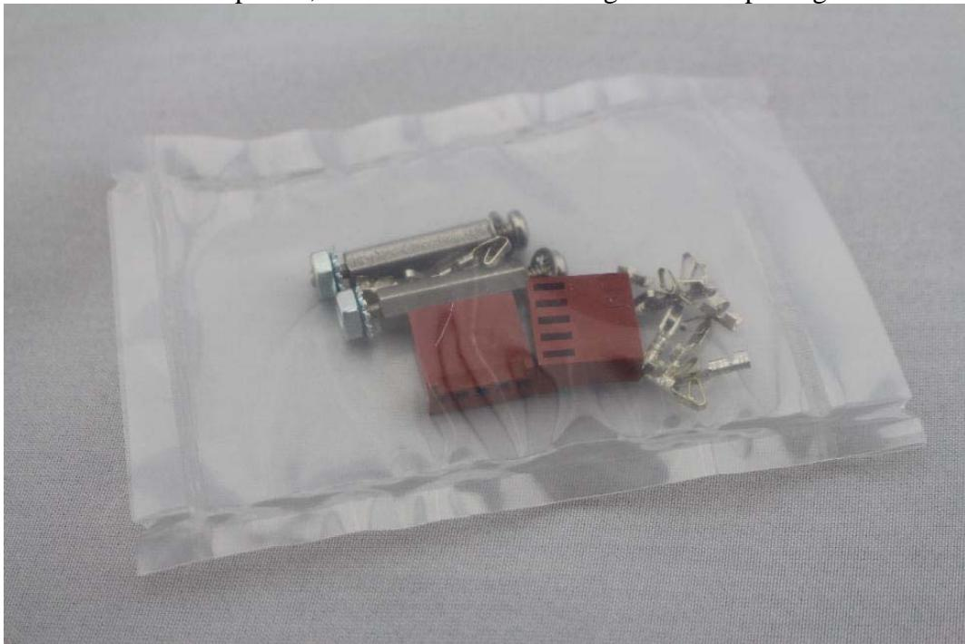
Attach spacers and lock nuts to Space Duel board at the places indicated below.
