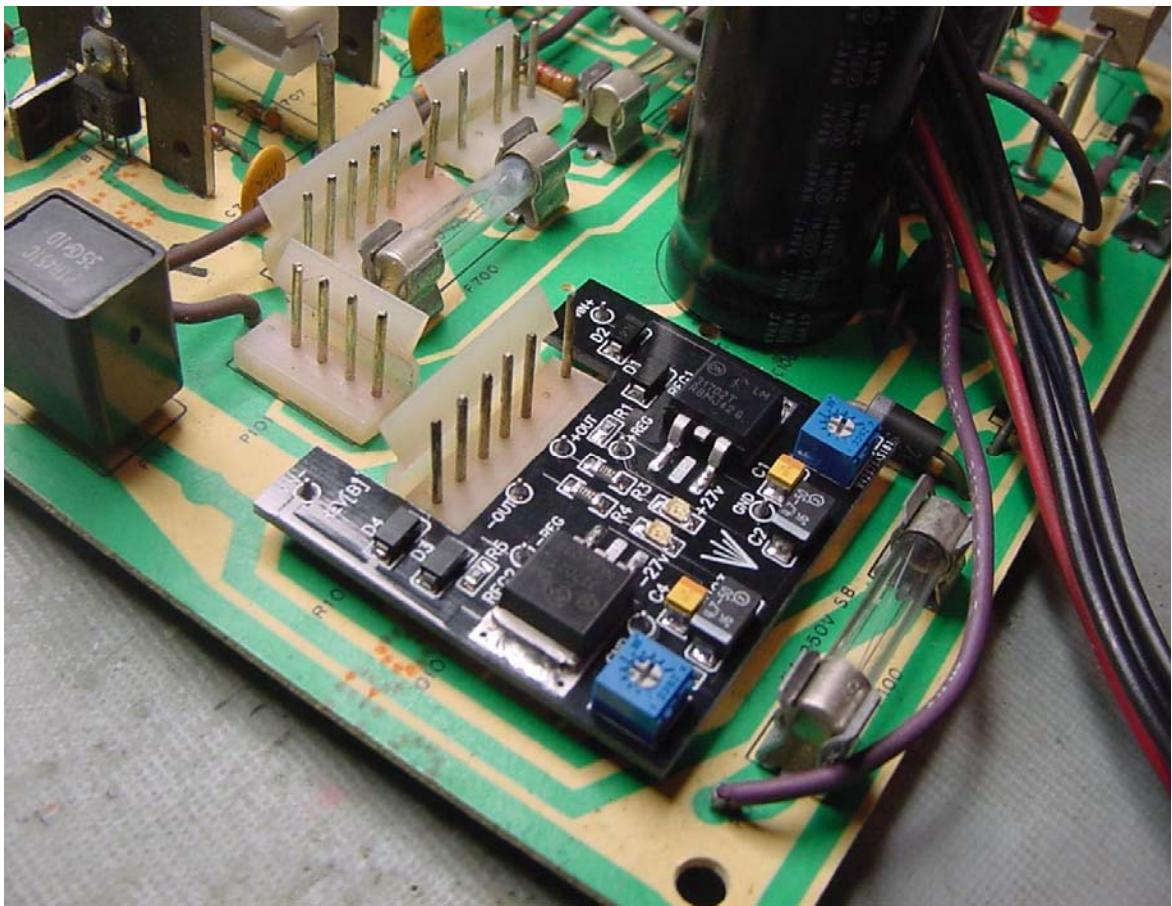
Insert PWB into deflection board as shown. Flip deflection board over and solder all pins. Board is factory adjusted but you can trim the voltages with the on board pots. There are +27v and -27V green leds to indicate power.
